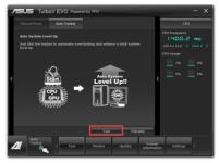
TurboV automatically overclocks the CPU, saves BIOS settings and restarts the system. After re-entering Windows, a message appears indicating auto tuning success. Click OK to exit.
