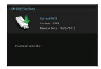
After you download the BIOS file to your flash drive, you can update the motherboard's BIOS. Refer to BIOS\_FLBK switch section in 2.2.6 Onboard Switches for details.
